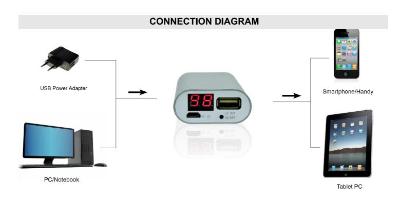
Please use the Mini / Micro USB cable to charge your LEICKE Portable Power Station.
